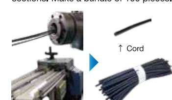
Extrusion and integrated cutting process 100 pieces: 1 bundle
